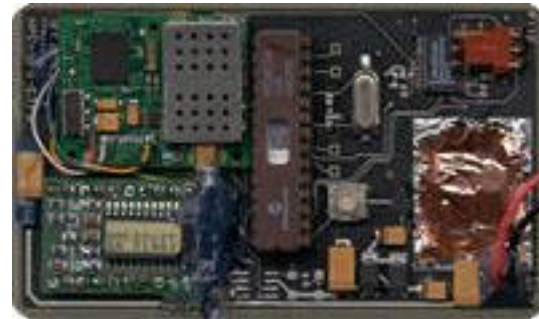
Prototype Websign client with magnetometer, GPS receiver, and the websign kernel
