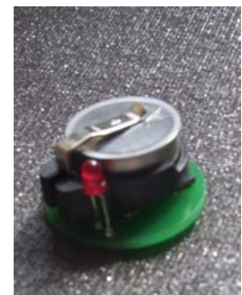
Figure 1. Left: diagram of a Pin&Play device accessing the network layers. Right: An actual Pin&Play pin attached to the surface. It holds a coin-sized unit (iButton) for memory and application specific processes, and an LED for basic user interaction.
