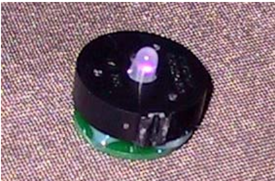
Figure 2. The Mixer Pin contains one multi-colour RGB LED, and three digital potentiometers that drive the red, green and blue values for the LED.
