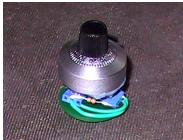
Figure 4. The Primary Pin contains a dial that is connected via a potentiometer to an analog-to-digital converter. It controls the intensity of one of three primary colours for the Mixer Pin.
