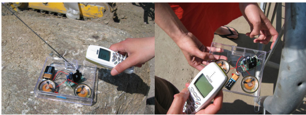
Figure 3: The two versions of Glitch: using a standard antenna and parasiting a metallic fence.
